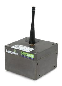
The GeoWAN Triaxial Tilt Sensor Node is an extremely high precision and exceptionally stable three axis tilt sensor which reports its measurements using Senceive's GeoWAN wireless communications network to a GeoWAN Gateway.
