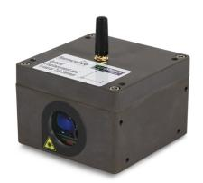
The FlatMesh Optical Displacement Sensor Node is an instrument which uses optical means to take high precision displacement measurements and pass these through Senceive's FlatMesh wireless communications network to a FlatMesh Gateway. It can also be combined with Senceive's world-leading triaxial tilt sensor to obtain high precision tilt measurements that are linked to an external reference.
