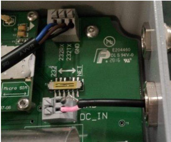
Figure. 110-240VAC to 12VDC@5A Adapter Connection.
