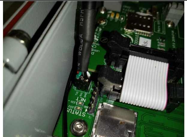
Figure. TTL to USB Connection.
