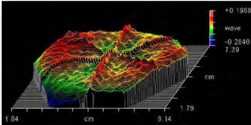
The above example shows a test measurement of the beam deviation for a round prism taken with an interferometer. Interferometer measurements determine phase in homogeneity, how well polished a particular prism is.
