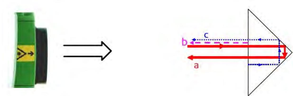
This part of the returned signal will disturb the desired signal because its travel time is shorter since it does not penetrate into the glass body of the prism.
