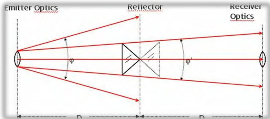
The distance measurement is based on the detection of the phase difference (or time of flight) between incoming and outgoing signals.
