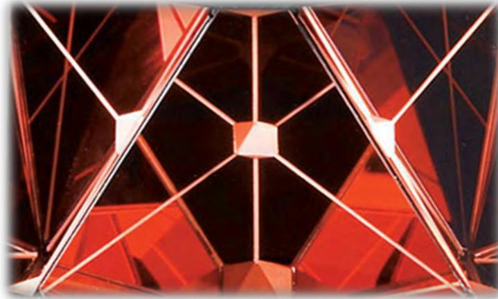
The degree of reflection of a surveying prism is defined as the ability of a material to reflect visible and infrared radiation. This capability depends on the material itself, as well as on the surface quality. To improve performance, reflex and anti-reflex coatings are often used. But what's the difference between the coating types, and how do they affect prism reflection?
