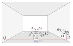
Afterwards turn the device exactly 180° around the plumb point P1 and position the right-hand perpendicular beam to the existing reference point a1. Make sure that the upper plumb point is still exactly on the reference P1. Then mark the lefthand beam to the right wall and mark it with c2. Finally measure the difference between the former reference point c1 and the new point c2. The deviation may be max. 3mm between these two points.
