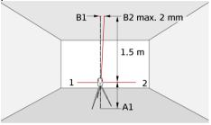
Rotate the instrument by 180° so that it points in the opposite direction 2 to direction 1. Adjust the instrument so that the laser beam hits point A1 exactly. If point B2 is no further than 2 mm away from point B1, then the Leica Lino is within tolerance.
