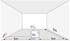
Place lock switch in "Unlocked" position (see Levelling lock). Mark a reference point (P1) approx. 5m from the walls and position the lower plumb point exactly on it. Align the cross hair to the left wall and mark the intersection point (a1) approx. on the same hight like P1 to the wall. Shortly after mark the right-hand perpendicular beam (b1) on the front wall.
