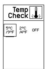
For each change in temperature of  $\pm$  5°C ( $\pm$  9°F) the Rugby returns to the level position to check if the change in temperature has led to a change of the main levelling system. For a more sensitive unit, you can change the setting to  $\pm$  2°C ( $\pm$  4°F) temperature change.
