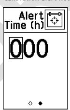
To be alerted of a calibration after X hours of use, enter the desired time before an alert appears.
