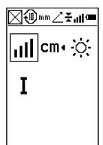
If there is no Rugby paired with the Combo a reduced menu screen is shown. This menu is limited to features that allow for the Combo to be used as a standalone receiver only.
