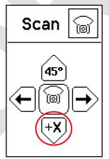
While in Scanning mode, the default direction of the scan is directly in the +X axis. Within the Scanning axis submenu, it is possible to redirect the scan to another axis.
