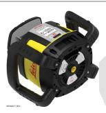
For layout work, use the Beam down mode to position the beam over a reference point. Then use the Scan mode to move the small scan quickly to a position to the left or right of the laser.
