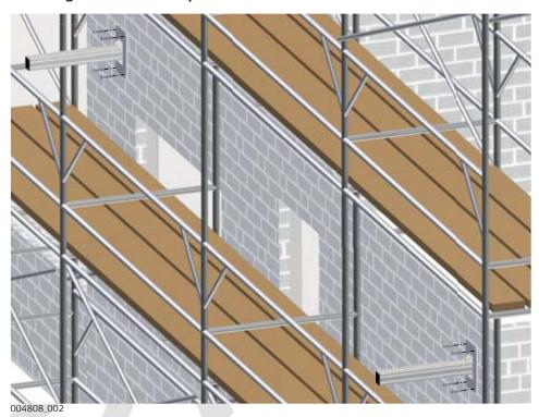
1. Mount the facade adapter brackets to the side of the building in locations where it is desired to have a laser and receiver setup.
