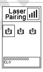
The Rugby and the Combo include radio modules that allow you to activate the functions on the Rugby remotely up to 300 m (1000') away.
