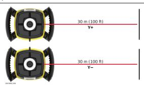
6. Align the second axis of the Rugby by rotating it 90° so that this axis is square to the wall. Allow the Rugby to self-level completely.
