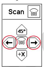
While in Scanning mode, the default direction of the scan is directly in the +X axis. Within the Scanning direction submenu, it is possible to control the direction of the scan manually.
