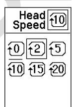
The currently active option is underlined. Press the OK/Grade button to select an icon. To navigate to the second menu page, press Right arrow/Volume button until page two is displayed.
