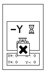
If the Rugby encounters a problem and the calibration process was not successful, the Rugby displays an "ERROR" screen for up to 2 minutes, then shuts off.
