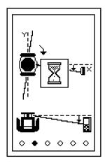
When the alignment procedure is successful, the Rugby displays the COMPLETE screen for 8 seconds, then resumes normal operation.
