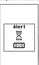
When the Rugby is re-levelling, the Temperature check wait screen is displayed. Wait until the process is finished before using the laser again. The Status LED flashes on the Rugby to indicate normal levelling.
