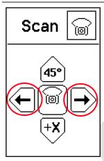
The scanning beam can be rotated using the left and right option on the Combo.
