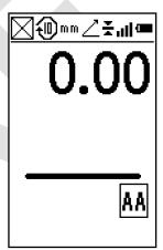
If the alignment procedure is not successful, the Rugby displays the ERROR screen for up to 2 minutes, then shuts down.
