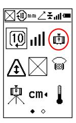
Press the Beam down option to check the alignment over a point.
