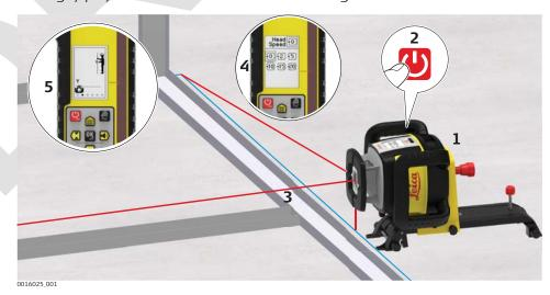
1. Attach the Rugby to the Smart Adapter and place in the laydown position.
