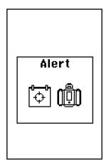
When the number of planned hours is reached, the calibration alert is displayed for 8 seconds. After calibrating the Rugby, the calibration alert hours are automatically reset. Changing or disabling the calibration alert is only possible by accessing the menu option "Calibration alert function".
