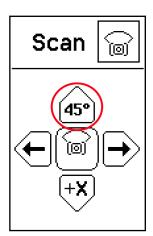
When installing suspended ceilings use the Combo to change to scanning mode for increased visibility.
