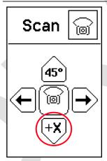
The scanning beam can be moved quickly in 90 ° increments using the Scan 90 ° option.
