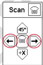
The scanning beam can be moved to the left or right side of the laser using the Scan 90 ° option.
