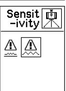
While levelling, the Rugby responds to disturbances, for example wind or vibrations, and stops the head rotation, if necessary. You can choose between two levels of sensitivity:
