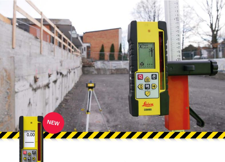
Laser receivers quickly and easily detect laser planes when the laser beam is not visible. Not only detecting the laser beam, they maximise performance of your Rugby laser and any construction laser on site. Work conveniently with Rugby lasers and Rod Eye receivers even at very long distances.
