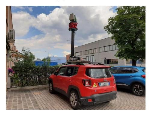
Lifting system for any brand and type of terrestrial laser scanner.
