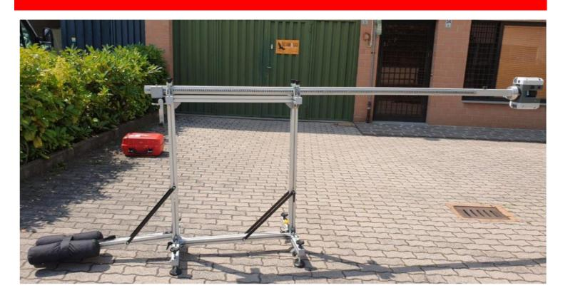
Horizontal extensible system for scanning with Leica RTC360, Trimble X7, TX5, Faro
