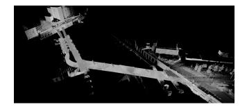
Detailed notes and photographs were taken using an iPad which were then geo-referenced to the point cloud assisting the data processing and production of deliverables. Data was then post-processed, and quality checked against the EDM survey ensuring the required accuracy was achieved. The required 3D topographical survey then produced a 3D AutoCAD file.
