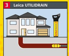
Use the Leica UTILIDRAIN to map pipes or sewers and find blockages. Use the Leica UTILIFINDER+ to trace the drain and obtain a depth reading.
