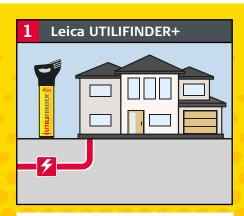
The Leica UTILIFINDER+ is a unique location system used to identify buried utilies. Select AUTO mode to detect loaded power cables.
