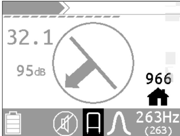
3. When fault probe is plugged into locator, locator will enter fault mode. Probe icon will show. A home symbol flashes in the bottom right corner of the locate screen.
