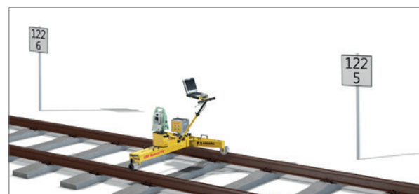
Relative track geometry survey with Amberg IMS 1000
