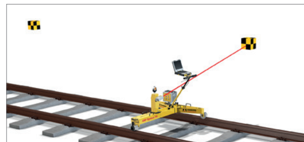
3D as-built survey with Amberg IMS 3000
