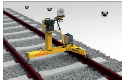
Absolute as-built track and infrastructure survey
