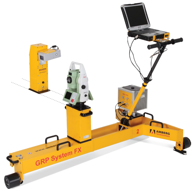
Front: Amberg IMS 1000 with tachymeter Back: Profiler 110 FX for Amberg IMS 3000
